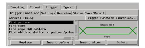
Trigger functions provide a simple way to set up the analyzer to *trigger* on common events and conditions. A library of functions is available for both *state* and *timing* measurements.
