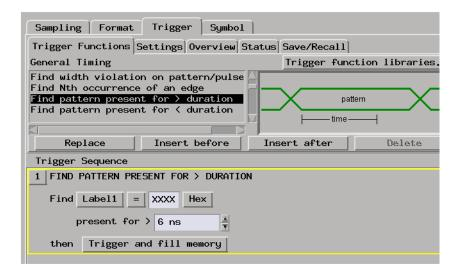
2. In the Trigger Sequence portion of the Trigger tab, select the buttons to define the label values and/or other conditions you want to trigger on.
