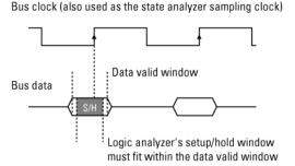
• Because the location of the data valid window relative to the bus clock is different for different types of buses, the position of the logic analyzer's setup/hold window must be adjustable (relative to the sampling clock, and with fine resolution) within the data valid window. For example:
