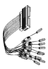
The standard lead set plugs directly into any .1-inch grid with 0.026 to 0.033-inch diameter round pins or 0.025-inch square pins. All probe tips work with the Agilent Technologies 5059-4356 surface mount grabbers and the Agilent Technologies 5959-0288 through-hole grabbers.
