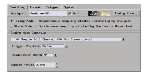
When you select Timing Mode, the Timing Mode Controls area appears.
